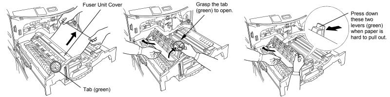
Figure 5.4. Paper jammed at the fuser unit
